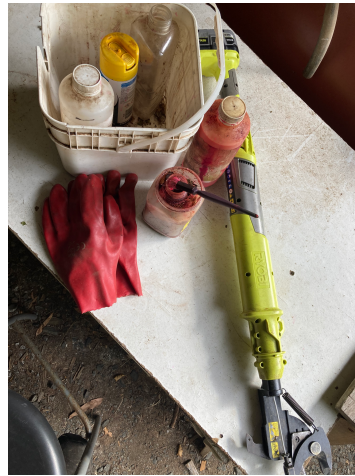
Image: Herbicide painting setup and cordless lopper
